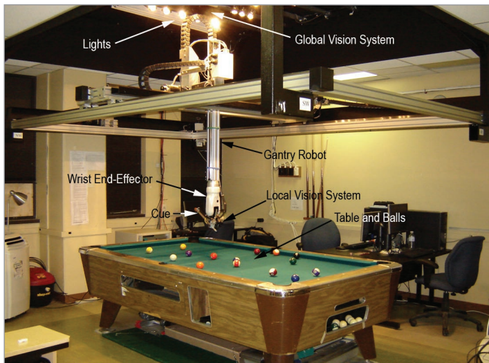
Figure 1. Deep Green robotic pool-playing system. The system is centered on a 3-degree-of-freedom gantry robot mounted to the ceiling to avoid impeding human access to the table.
